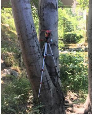
Image 9: Self-leveling Laser Set-up
