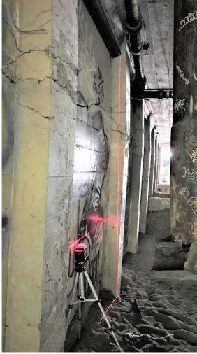
Image 12: Self-leveling Laser at Interior Pilaster
